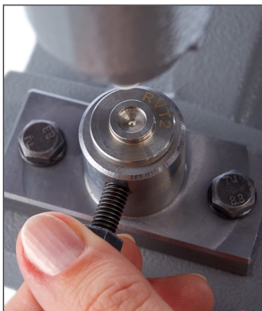
4. Tighten the lower die.
