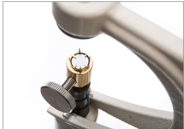
2. Put the pin into the upper die.
