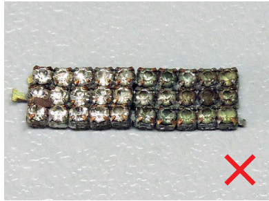
Stones damaged by long soldering and high temperature.
