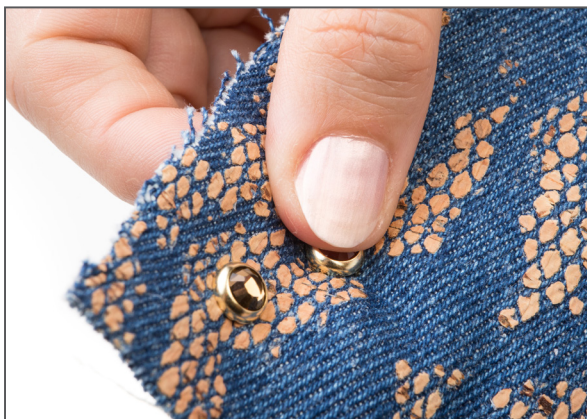
3. Push the prongs through the fabric.
