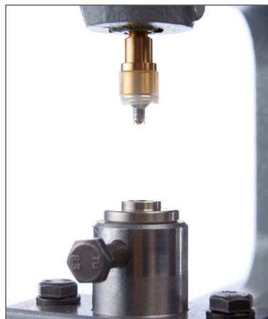
5. Attach the rivet to the upper die.
