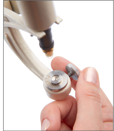
3. Tighten the lower die.
