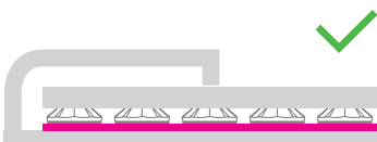
Plates are parallel - correct!
