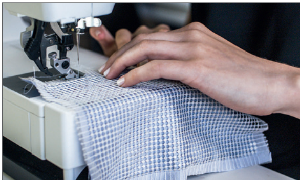
3. End sewing with backwards motion as with any textile.
