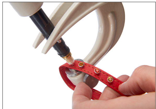
7. Applied Rivets on a leather band.
