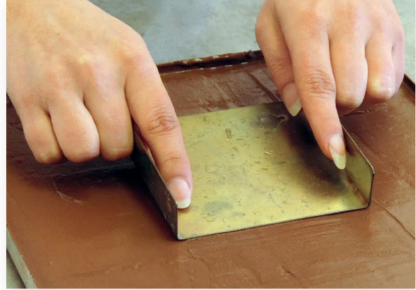
2. Spread the impression paste in the plate; smooth into an even and compact layer.
