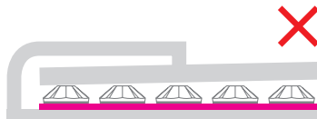
Plates are not parallel - incorrect!
