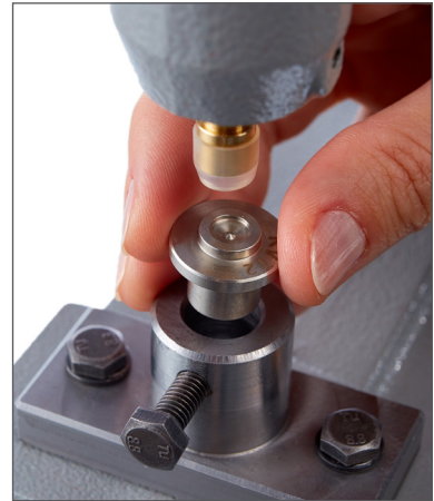
3. Placement of the lower die.
