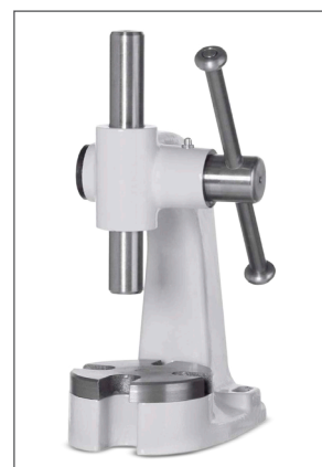
A fly press represents an easy way how to mechanically apply the products.
