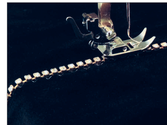
Detail of a zigzag stitch.
