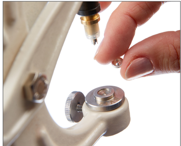
5. Place the back side of the Rivet on the lower die.
