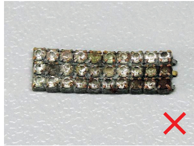
Stones damaged by long soldering and high temperature.
