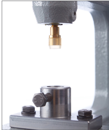
2. The upper die needs to be screwed in tightly.
