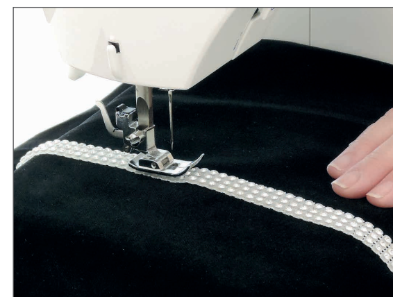
Multi-row banding and similar products are sewed on between the rows of stones.
