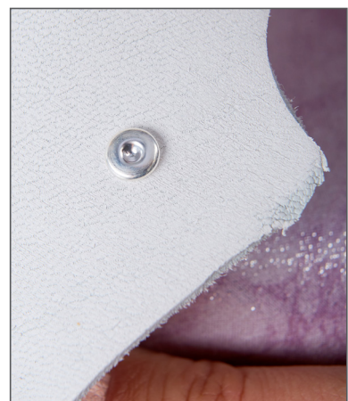
9. Applied Rivet from the bottom.
