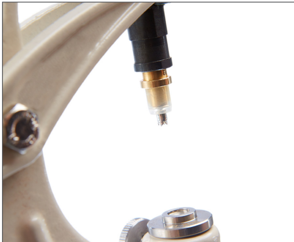
4. Attach the rivet to the upper die.
