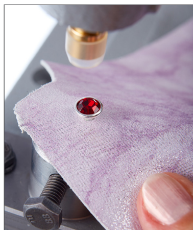
8. Applied Rivet from the top.
