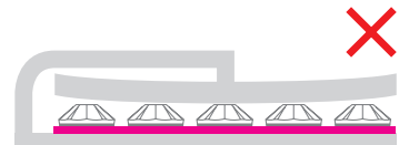
Plates are not parallel - incorrect!
