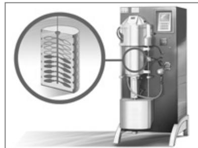
6 A casting machine next fills the investment with a choice of liquid metal (gold, silver, brass or alloys). By using pressure from above and vacuum from below, the casting machine not only ensures that the metal quickly fills the empty space but also that no air bubbles remain within the newly cast jewelry pieces.
