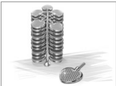
7 After casting, four hours are needed for the crucible to cool down to room temperature. The crucible is then quenched in water, also at room temperature, to dissolve the investment. The remaining metal tree is then jet cleaned with water before it is acid cleaned, for example with a 20% phosphoric acid solution.
