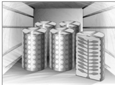
5 The crucible is heated in an oven, the burn out furnace, to melt and 'burn out' the wax. There is now empty space where the wax tree used to be. Only the investment remains.
