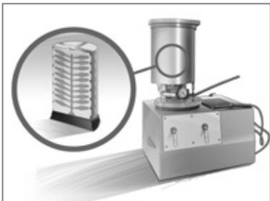
4 The wax tree is placed in a crucible. A machine is then used to inject investment, usually plaster, into the space surrounding the wax tree.
