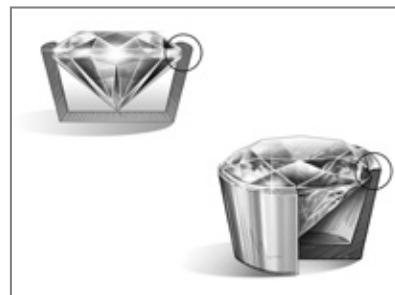
1 In preparation, a strip of metal is bent into the exact shape and size of the selected stone. After the stone has been inserted into the cavity, a setting tool is used to press the metal strip onto the stone. The metal strip is now bent over the edge of the stone.
