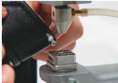
5 Now the 3D Stud is applied evenly and close to another 3D Stud.
