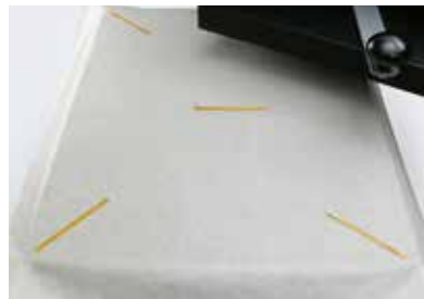
Test with temperature measuring strips (art. 9010/007)
