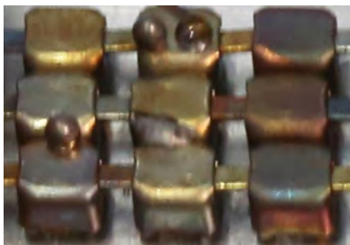
2 Too high temperature
